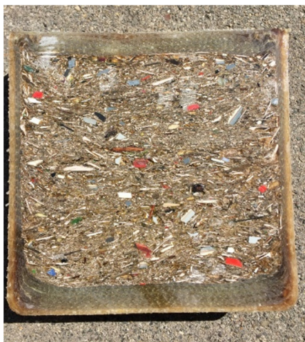
FIGURE 6 Cross section of guiding beam made of EoL composite.
